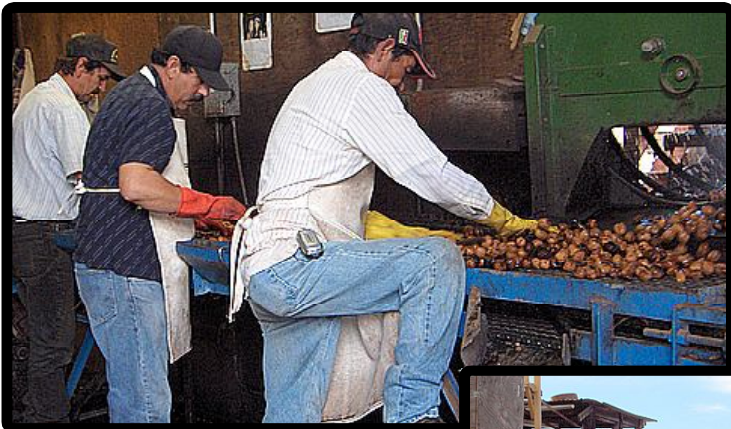
After debris is removed, nuts are rolled to remove the remaining hulls and any small debris
