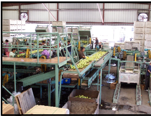
SIZER, SORTS BY WEIGHT OR SIZE SO PACKED BOXES HAVE THE SAME SIZE PEARS
