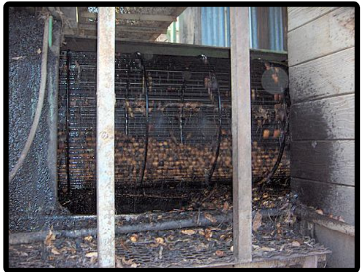
After debris is removed, nuts are rolled to remove the remaining hulls and any small debris
