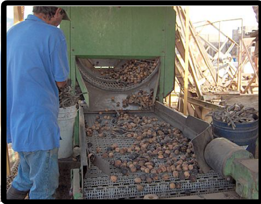
Nuts being cleaned of debris
