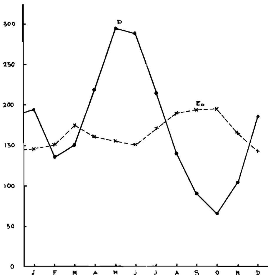
Fig.2. Average monthly precipitation (P) and free water evaporation (E<sub>o</sub>) at Republiek, for the years 1906-1972 except 1912 and 1957.
