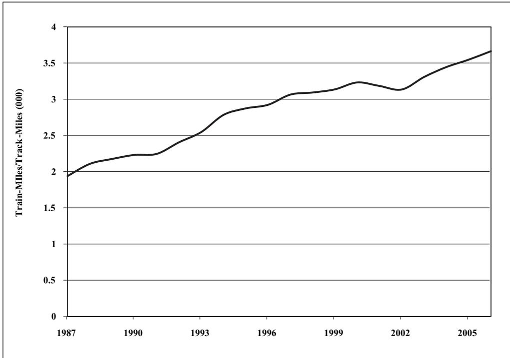
While density is beneficial, additional capacity may be needed as traffic grows. A study by Cambridge Systematics, Inc. (2007) indicates that 12% to 13% of U.S. rail lines are at or near capacity. Another 39% have volume/capacity ratios of 0.4 to 0.7. With continued traffic growth, 45% of U.S. rail lines are projected to be near, at, or beyond capacity in 2035 without expansions (Cambridge Systematics, Inc. 2007).
