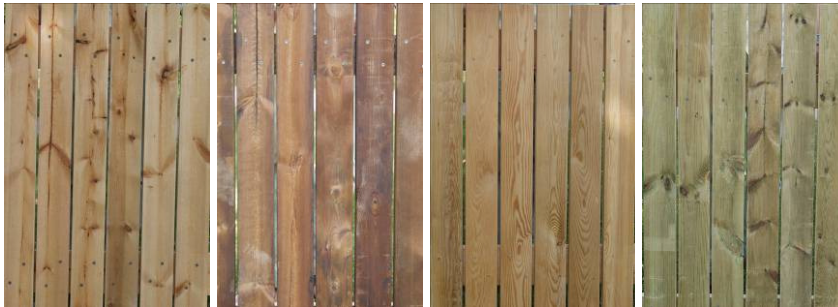
Figure 2. Deck material samples used in the study (left to right: organic biocide treated pine, furfuylated pine, untreated Russian larch, copper treated pine).
