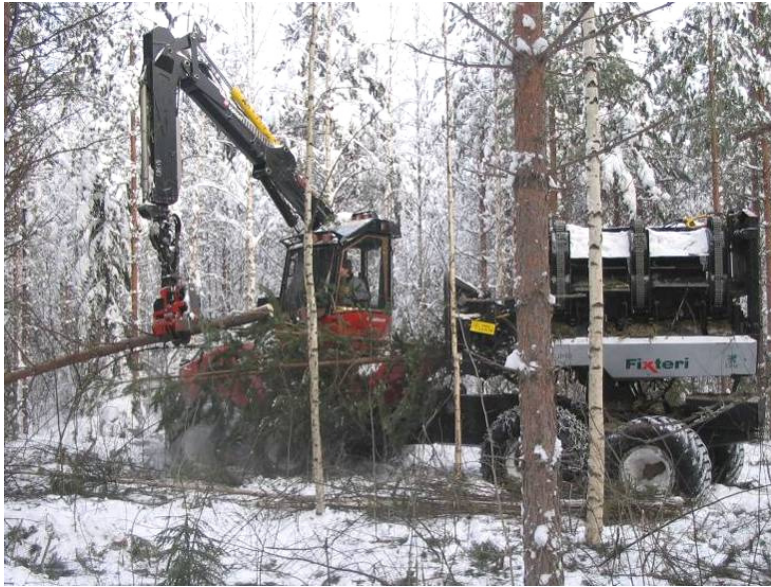
Figure 1. The first prototype of the Fixteri whole-tree bundler taking wood onto the feeding system of the bundler. Photos: Metsäteho Oy / Kalle Kärhä.
