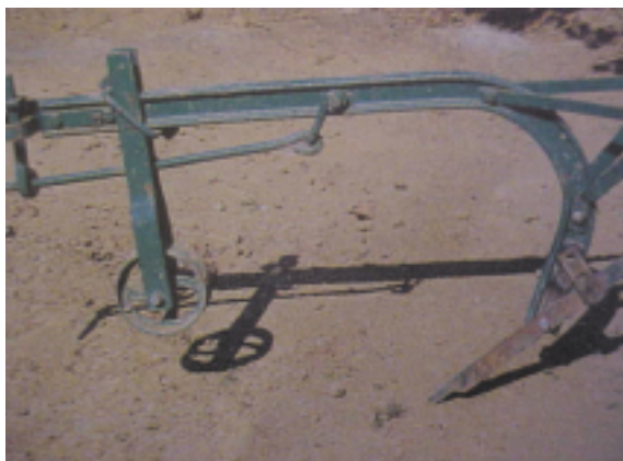
Picture 13: A subsoiler – equipment used to break the hard layer in the soil
