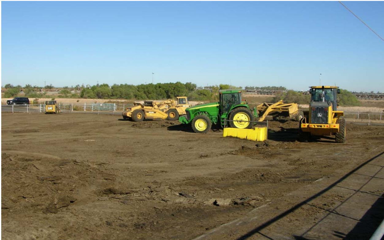
Figure 1. Manure harvesting using a tractor-pulled box scraper, front-end loader and elevating scraper. Source: Dr. Brent Auvermann, Texas AgriLife Research and Extension Center at Amarillo.
