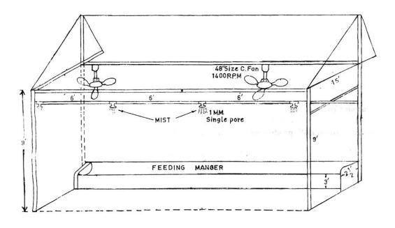
Figure 1. Design for Mist and Fan system
