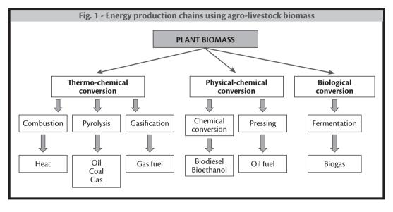
In particular, the term biogas refers to a mixture of gases, consisting primarily of methane (50-80%), obtained from the anaerobic fermentation of biomass of plant and animal origin.
