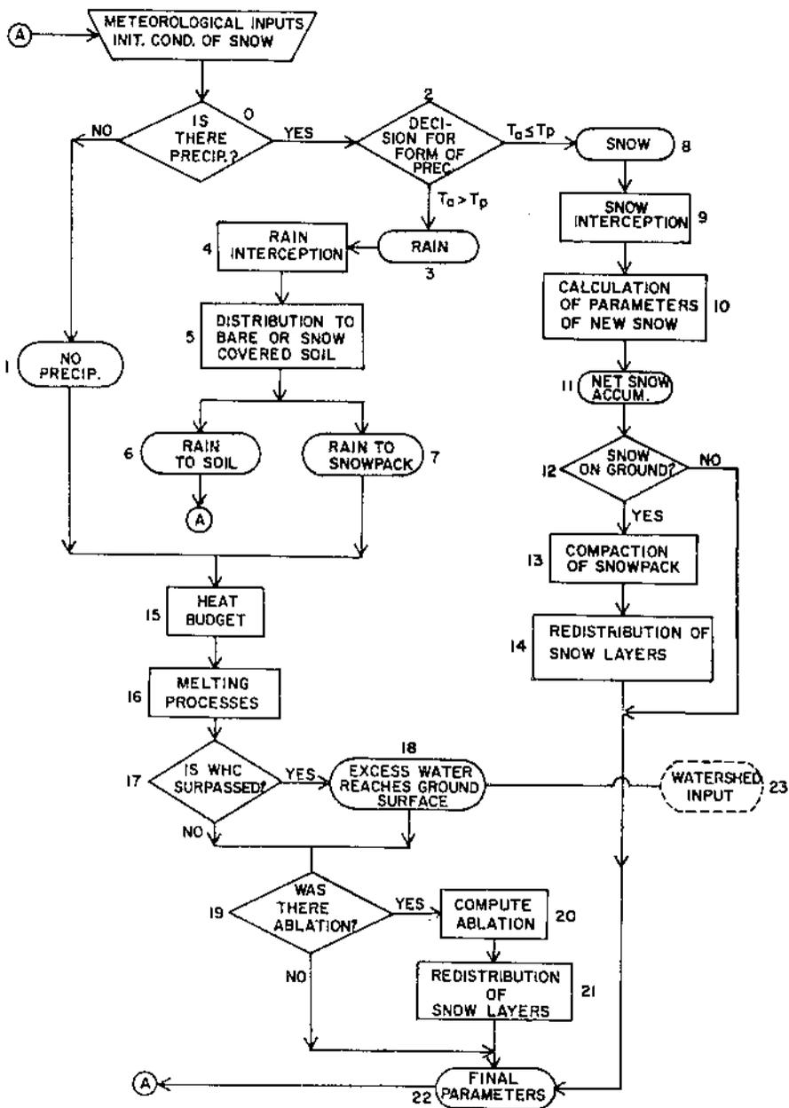
FIGURE 7-3.—Simulation of snowmelt.
