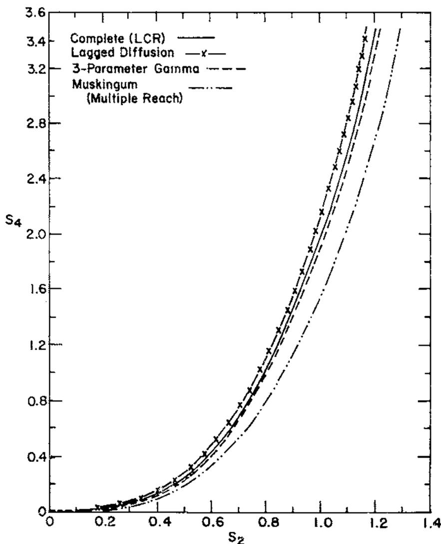
FIGURE 9-11.—Shape factor diagram for three-parameter model ( $F=0.5$ ).
