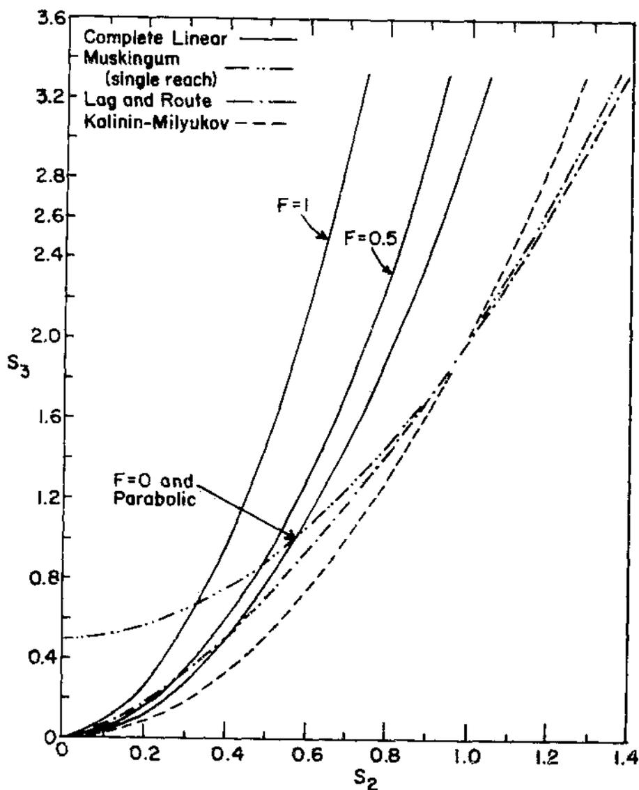
FIGURE 9-9.—Shape factor diagram.
