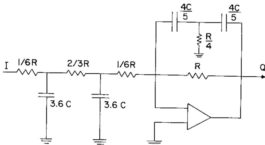
FIGURE 7-13. --Direct analog for distortionless linear channel.
