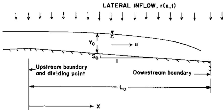
FIGURE 9-1.—Overland flow (two-dimensional).
