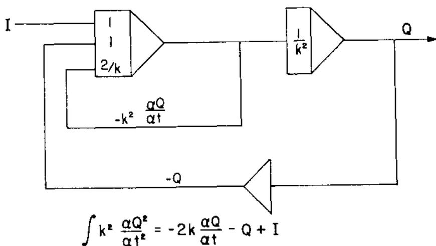
FIGURE 7-10. —Indirect analog for two linear reservoirs in series.
