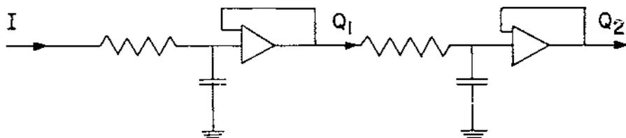
FIGURE 7-12.—Direct analog two linear reservoirs.
