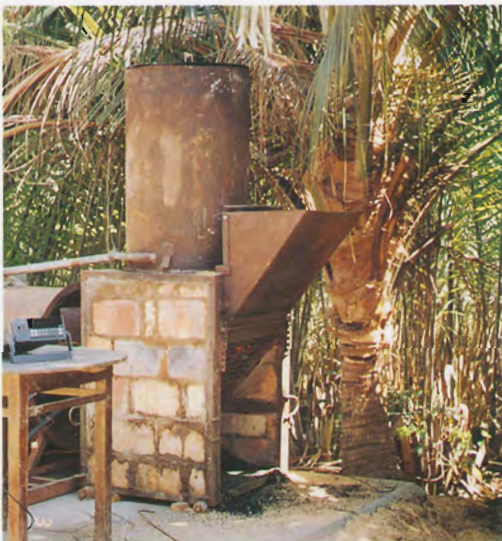
Figure 3. Inclined grate furnace with cyclonic ash separator.
