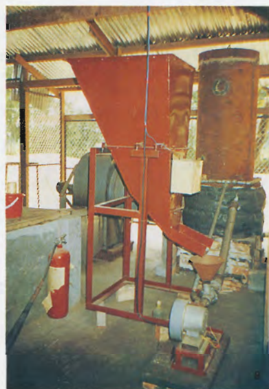
Figure 8. (a) the 80 t in-store dryer at Song-Hau Farm, 1994; (b) rice-husk furnace with pneumatic feeder and cylindrical combustion chamber, used as heat source for the 80 t in-store dryer.
