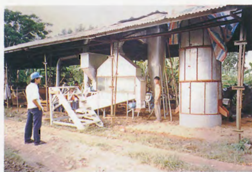
Figure 1. The 1 t/hour fluidised-bed dryer fabricated at the University of Agriculture and Forestry, Ho-Chi-Minh City.
