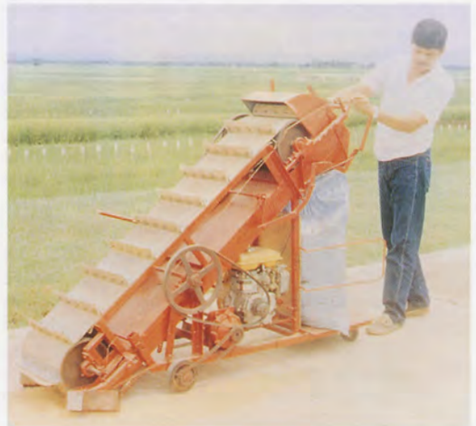
Figure 1. The pavement grain collector designed by IRRI.
