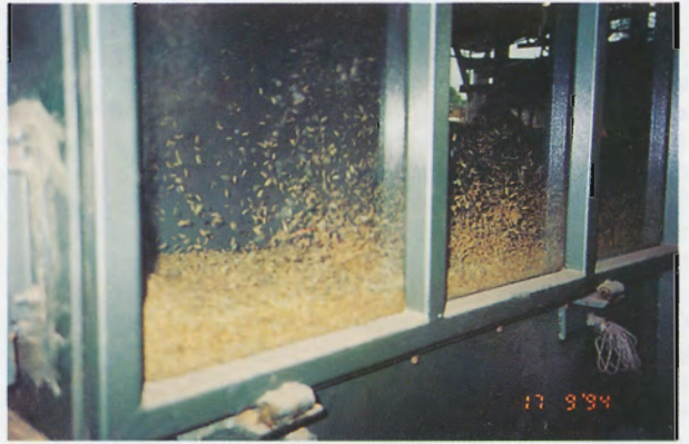
Figure 7. Prototype 1 t/hour fluidised-bed paddy dryer.
