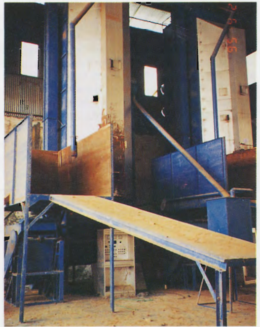
Figure 1. Flat-bed batch dryer of 10 t capacity at a seed processor in West Java. (below)
