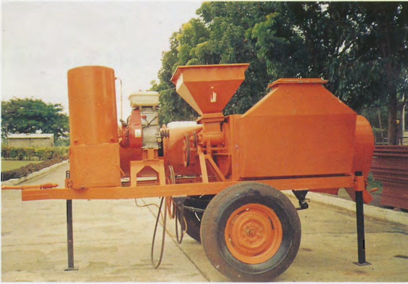
Figure 7. The prototype model of the rotary semi-fluidised system dryer.
