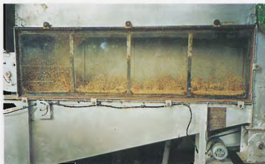
Figure 9. Fluidised-bed dryer at Song-Hau Farm, September 1995.
