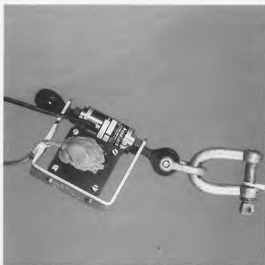
Fig. 2. Load cell with inclinometer, allowing force to be measured together with the corresponding angle of pull.
