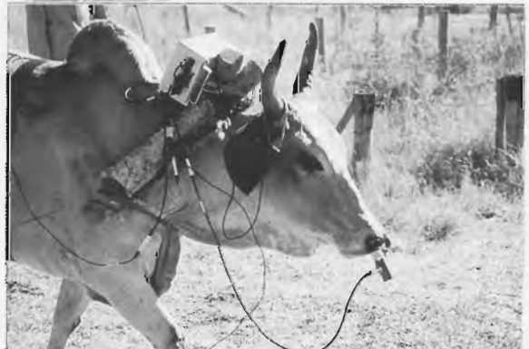
Fig. 1. Modular system in use with breathing rate and heart rate sensors attached (ILCA, Ethiopia 1988).
