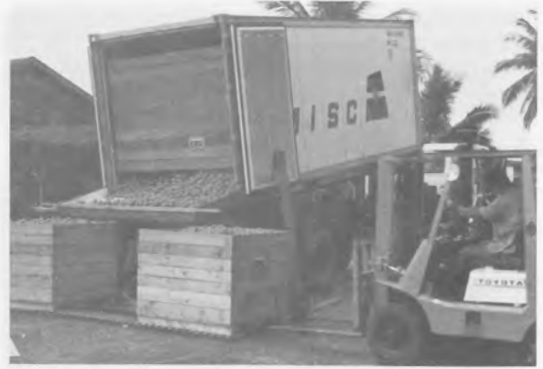
Fig. 4. Simple hopper for unloading bulk oranges.
