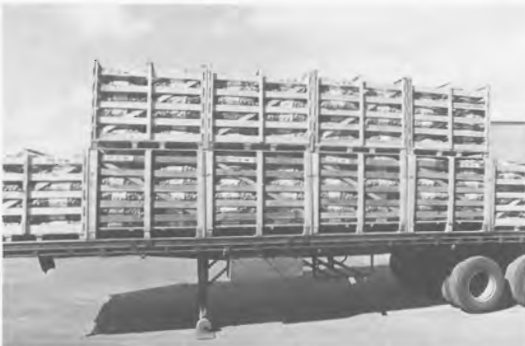
Fig. 2. Wooden pallet bins used for carrying onions in the ventilated vehicle decks of roll-on-roll-off ships.
