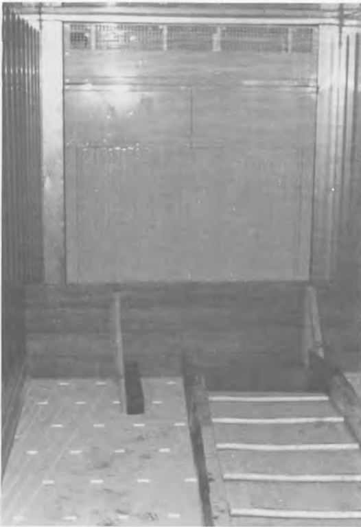
Fig. 3. Temporary baffle inside container.
