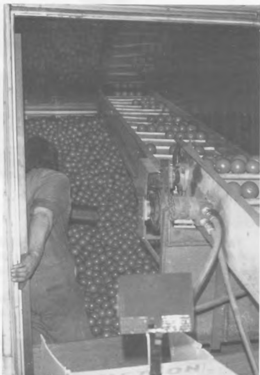
Fig. 1. Conveyor filling container with oranges.
