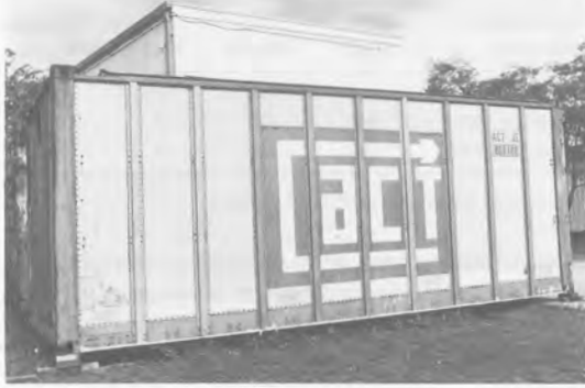
Fig. 5. Fantainer showing evenly spaced inlet vents in the side wall.
