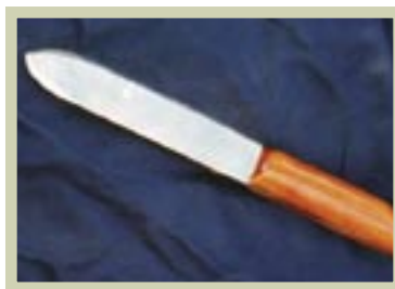
Figure 7-5. Coconut knife, designed with sufficient weight to crack open the dehusked nut and remove the kernel in strips.
