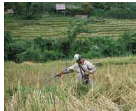
Figure 7.3 Radio-tracking with a three-element, folding 'Yagi' antenna.
