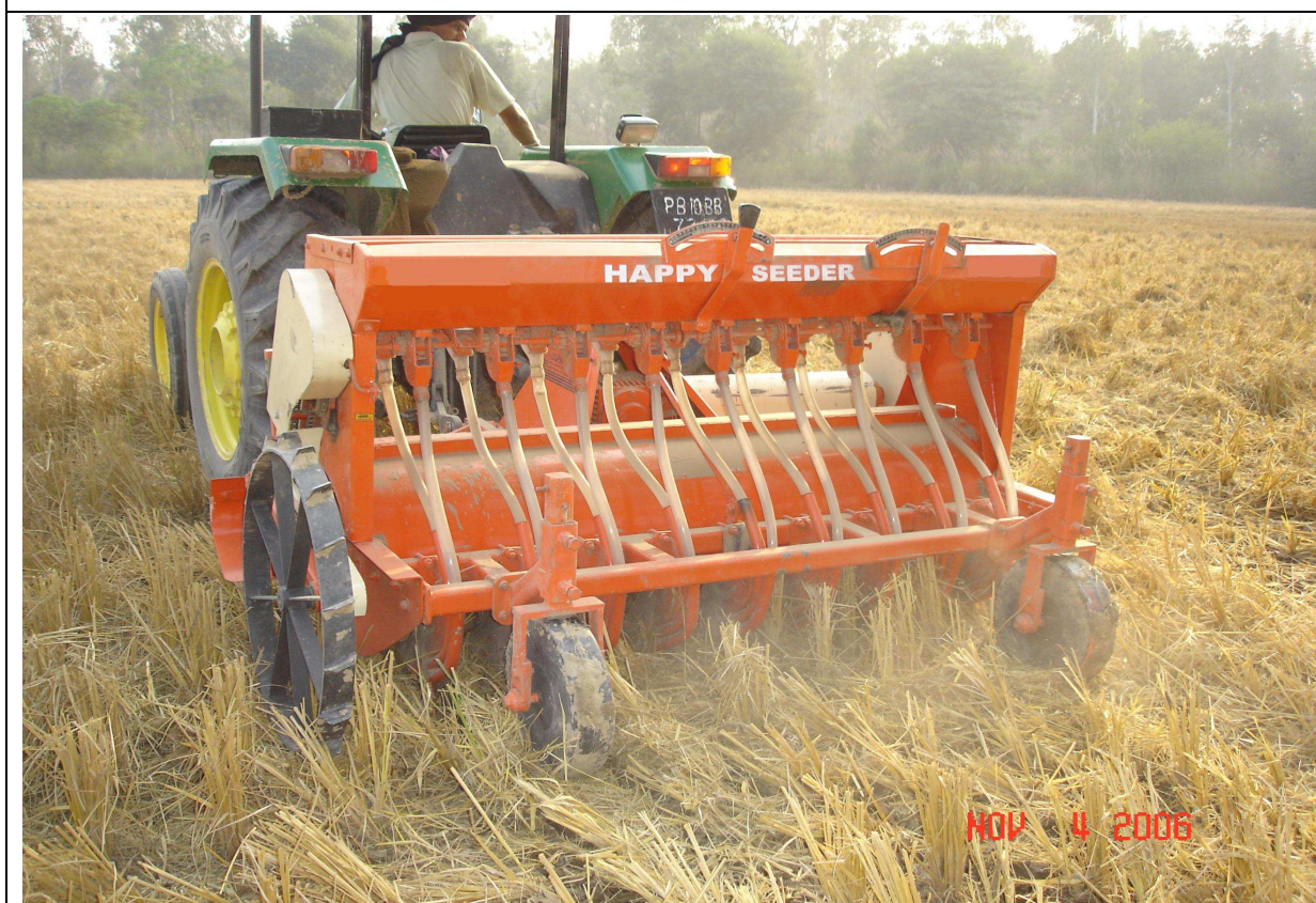
Figure 4: The Happy Seeder Direct Drilling Wheat in Standing Rice Stubble
